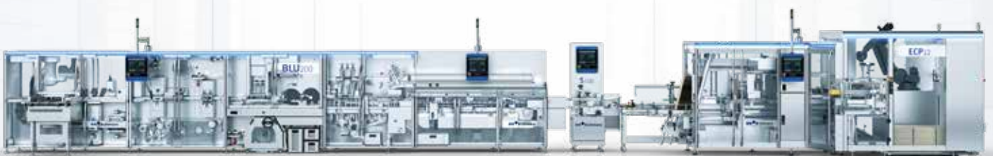
Packaging line of parenteral products with Uhlmann Track & Trace: unique identification and traceability with medical device tracking in the blister machine, printing system and camera inspection in the cartoner, S 500 for serialization, and aggregation in the end-of-line packaging machine
